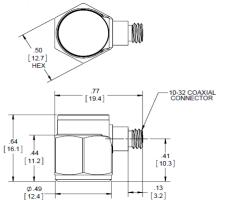
Units on the line drawing are in inches, units in brackets are in millimeters. Refer to 127-3055DT for more information.
